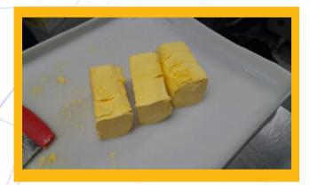
A root cause analysis was done on the inconsistency of weight of butter products packed coming from the machines. Examples of rejected product are shown in the photo. Reasonss for rejection include tear marks on the side of the butter.
